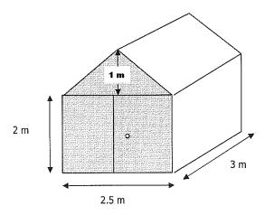
8. A) The diagram below show the outside dimensions of a partially finished factory building.
